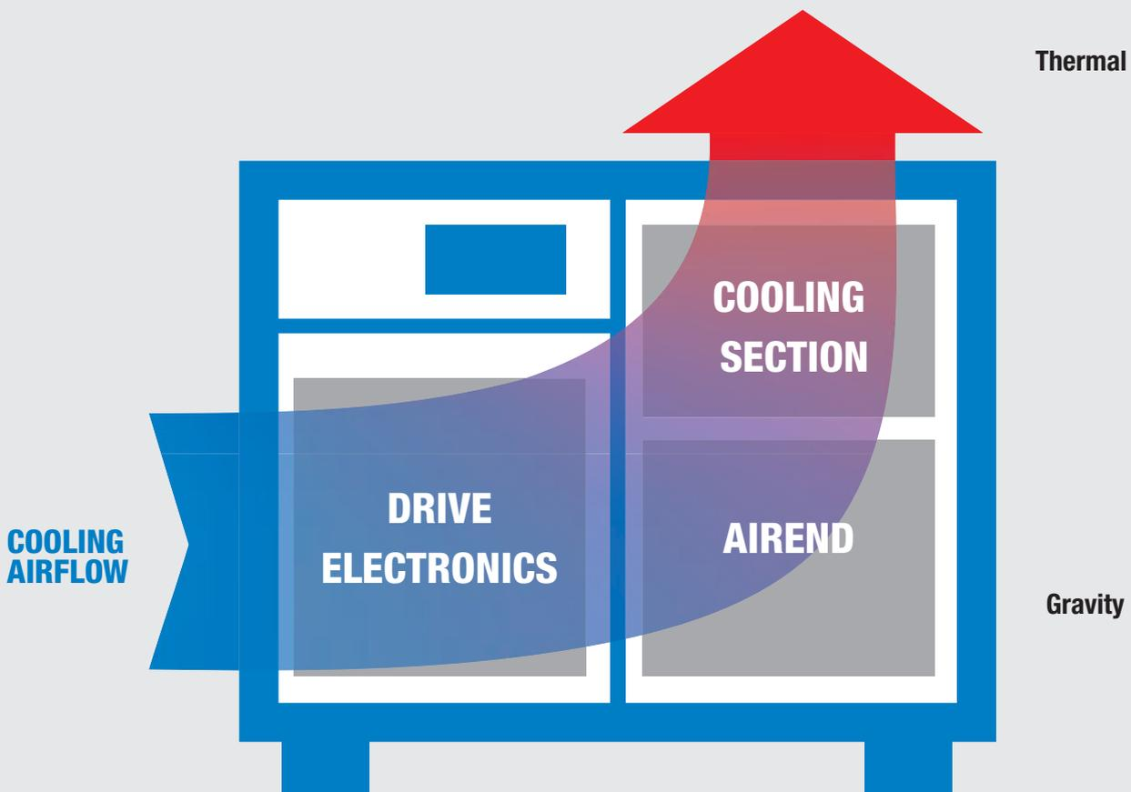
**Intelligent engineering from BOGE:** The three main sections of the BOGE screw compressor (electronics & drive, compressor, independent cooling unit) are strategically aligned in the main cooling air flow: for maximum efficiency and service life.
