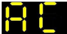
Digital display indicating Alarm Cycle
